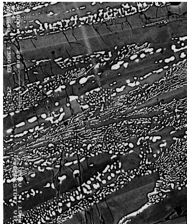
Fig. 1. SEM micrograph of as cast \text{Re}_{27}\text{Al}_{73} showing primary \text{Re}_4\text{Al}_{11} + eutectic ( \text{Re}_4\text{Al}_{11}+(\text{Re}) ).
